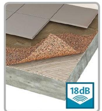
V-notched trowel, apply acrylic glue to the concrete slab. Gently, return the pulled back material to its measure place and roll in both directions with a roller. Proceed to cover the entire floor making sure that the joints are butted tight. After completion, the AcoustiCORK T66 should cover the entire flooring area without gaps and with joints securely taped.
